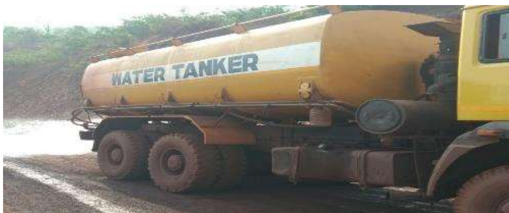
Photo-1: Mobile Water Tanker for dust suppression on mines haul road
